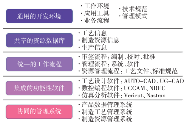
图1 集成数控加工工艺准备应用平台规划 Fig.1 Application platform planning of integrated numerical control machining process preparation
